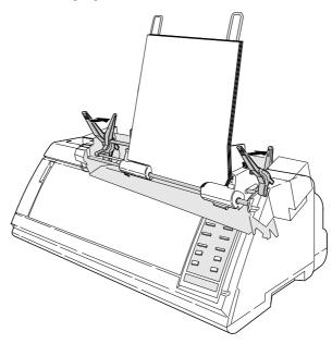
**11.** Press the PAPER PATH key to select CSF FRONT or CSF TOP.
